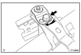
(b) Remove the No. 2 tilt lever lock bolt and No. 1 support reinforce.
