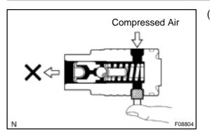
(b) Check the flow control valve for leakage. Close one of the holes and apply compressed air of 392 - 490 kPa (4 - 5 kgf/cm<sup>2</sup>, 57 - 71 psi) into the opposite side hole, and confirm that air does not come out from the end hole.
