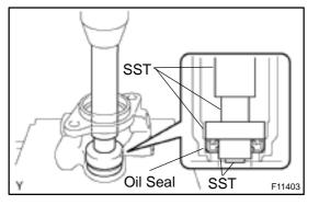
(c) Install the oil seal to SST, and press them into the rack housing.
