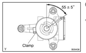
(b) Install the reservoir with the clamp to the position shown in the illustration.
