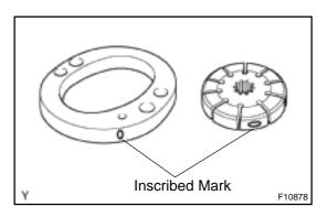
If it is more than the maximum, replace the vane plate and/or vane pump rotor with the one having the same mark stamped on the cam ring.
