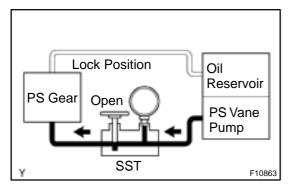
(g) With the engine idling and valve fully opened, turn the steering wheel to full lock.
