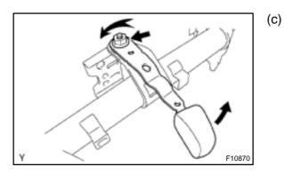
Install the adjusting nut by rotating it counterclockwise in the specified torque so that the locking load (load applied to when a knob is operated) of the tilt lever will be 38 – 82
