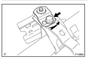
(d) Install the No. 1 support reinforce with the No. 2 tilt lever lock bolt by turning it counterclockwise.
