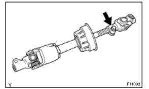
11. REMOVE SLIDING YOKE AND NO. 2 COLUMN HOLE COVER
